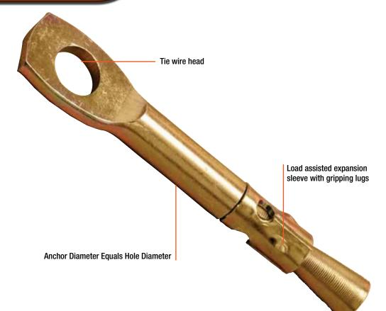
The TruFast<sup>™</sup> Push-Pull Suspension Anchor is an all metal, tie wire, load assisted expansion anchor designed for fixing suspended ceiling cables to concrete soffits.
