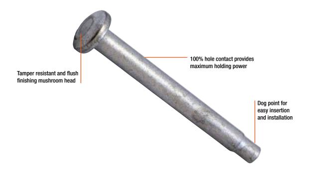
The RediDrive<sup>™</sup> Hammer-In Anchor is a one-piece, all steel, light duty, impact setting, interference fit anchor designed for use in concrete. The RediDrive<sup>™</sup> is simply hammered through the fixture into a pre-drilled hole. Its tamper resistant mushroom head sits flush and its interference fit is permanent.
