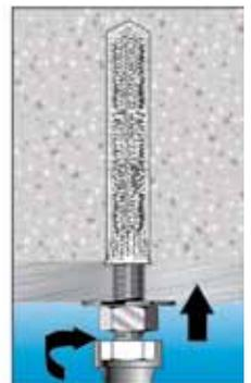
14. Attach fixture and tighten nut in accordance with recommended tightening torque.
