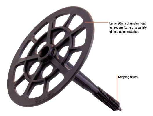
The InsulFast<sup>™</sup> Drill Anchor is a light duty, impact set, interference fit anchor, designed for fixing the majority of insulation materials to solid substrates such as concrete, brick, block and stone.
