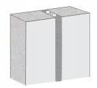
Up to 4 hours Fire Rating Vertical Joints (2 Sides Sealed) • FyreBrake<sup>™</sup> Sealant with backer rod
