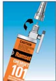
7. Mount assembled cartridge into the Ramset Universal Applicator (Mount Ultrafix™ Plus in regular caulking gun).
