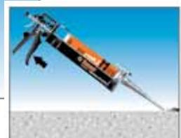
9. Insert mixer nozzle to the base of the hole and inject.
