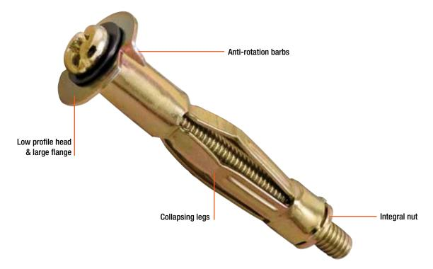
The Ramset<sup>™</sup> Hollow Wall Anchor is an all metal, light duty, cavity fixing for plasterboard and other hollow wall materials up to 38mm.
