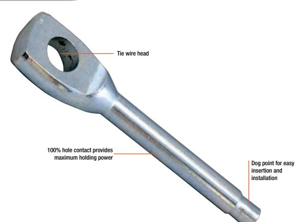
The Ramset<sup>™</sup> Catenary Wire Eye is a one-piece, all steel, light duty, impact setting, interference fit suspension anchor designed for use in concrete soffits. The anchor is simply hammered into a pre-drilled hole where its 100% interference fit is permanent.
