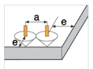
• The coincidence of stress cones of adjacent anchors in concrete reduces their tensile performance.
