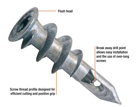
The WallMate<sup>TM</sup> is the original self drilling plasterboard anchor. Available in nylon or zinc, the WallMate<sup>TM</sup> would probably be the quickest and easiest plasterboard anchor to install and remove.
