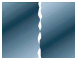
Typical interference fit has 30% metal-to-metal contact.
