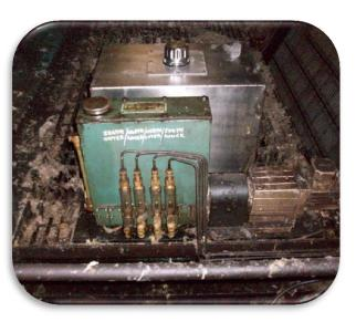
Rotalube replaced oil spit/spray system on Forming oven saving \$80K Per year in oil. Rotalube replaced PDU spit system (as shown) on a 6 inch pitch, forming oven chain.
